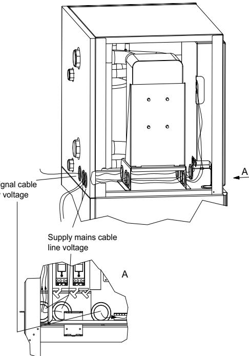
Fig. 7.4:Cable inlet switch box
